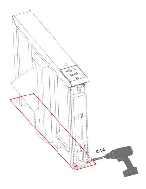
6. Clean up the soil and dust after the drilling is completed, place the turnstile to the installation site again.
