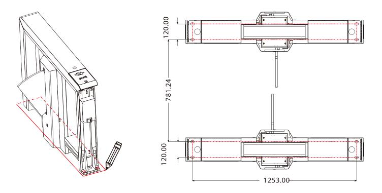
5. Take the turnstile aside and use the electric drill according to the drawn screw holes.
