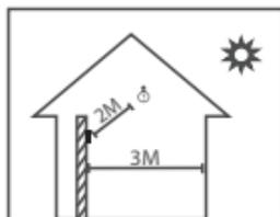
Install the device indoors at least 10 feet (3m) away from window, and 6.5 feet (2m) from light source. It is not recommended to install on the windows or in outdoor.
