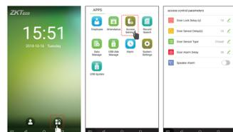
Go to Main Menu > **Access Settings** > **Access control parameters** to enter **Access control parameters** setting interface.
