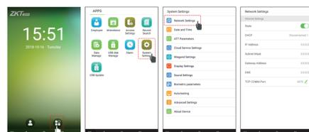
Go to Main Menu > **System Settings** > **Network Settings**, set the IP Address. The device will communicate with PC via the Ethernet parameters. Using Cloud Service Settings sets Server Address and Server port according to the server.
