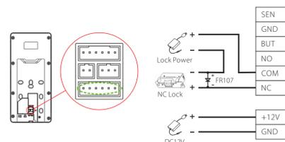
◆ Device sharing power with the lock is shown below:
